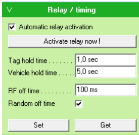
Figure 27: Relay / timing settings
