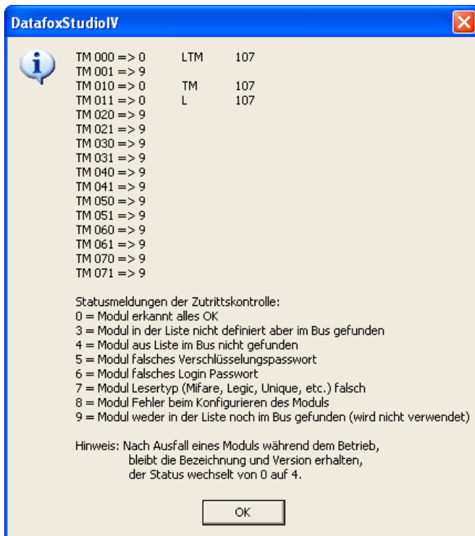
Figure 83: State of ZK-module
