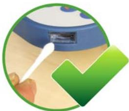
Impure laser scanning windows have to be cleaned to keep up the functionality. Use cotton swabs and water, or a gentle cleanser (no **scrubbing solution** or **acidic cleaner**) to clean the window. Never use **pointy** objects for cleaning. This may scratch the scanning window and effects the functionality of the laser.
