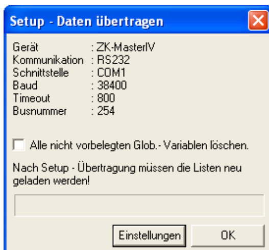
Figure 76: Transmitting setup data
